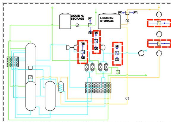
Figure 2: Scheme of Air Separation Unit with highlighted potential for WHR
