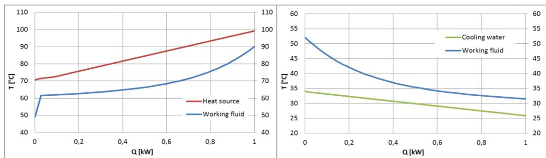
Figure 10: Q-T diagrams with temperature match of heat input and rejection for LiBr Absorption Power Cycle
