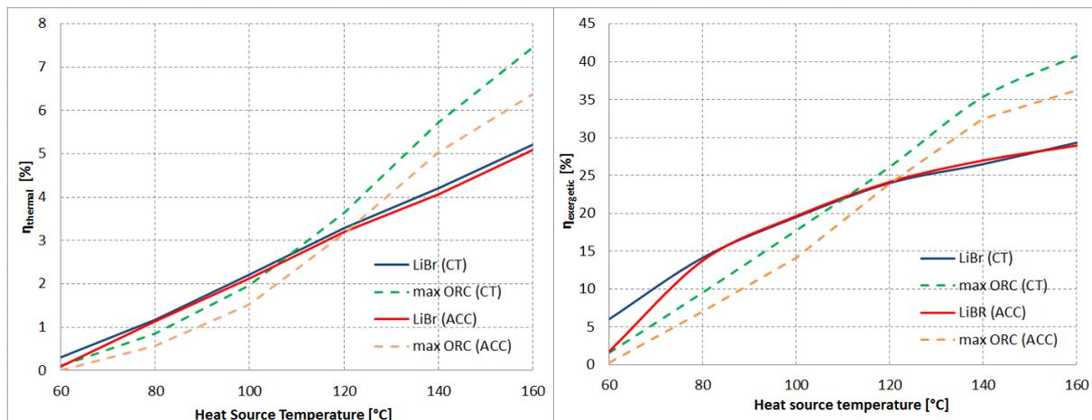
Figure 11: Thermal and exergetic efficiency WHR systems of maximum from range of ORCs and LiBr based absorption power cycle with cooling by wet fan cooling tower (CT) and Air Cooled Condenser (ACC)
