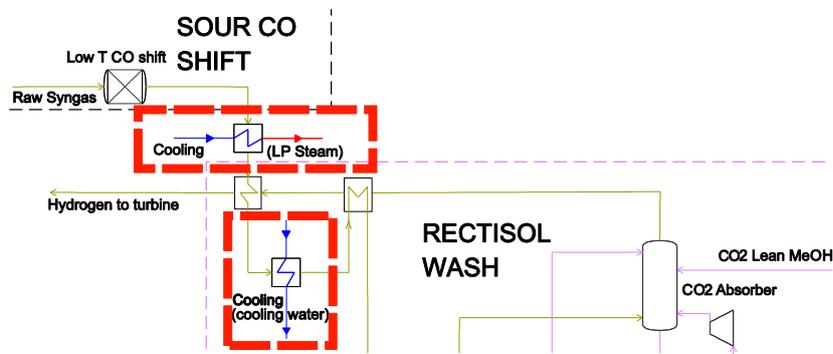
Figure 4: Syngas node between CO Shift, Rectisol wash and turbine
