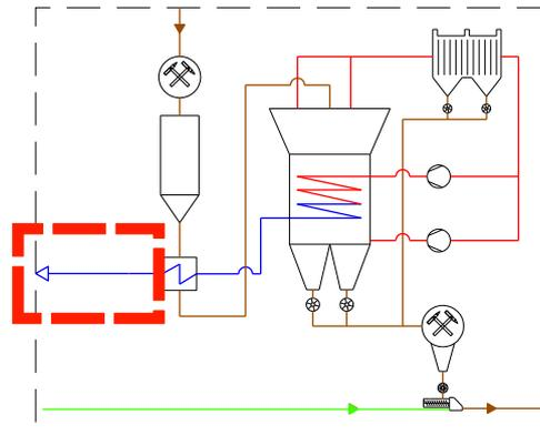
**Figure 3: WTA fluidized bed dryer with highlighted waste heat stream**
