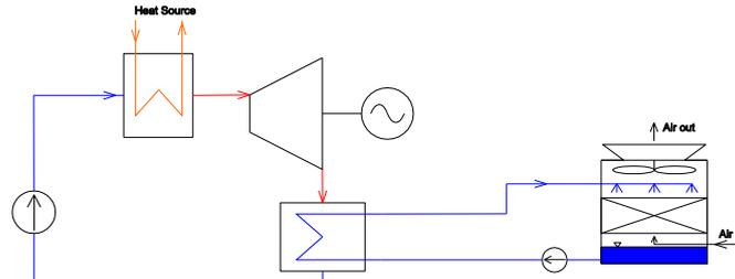
Figure 8: Basic scheme of the ORC WHR system
