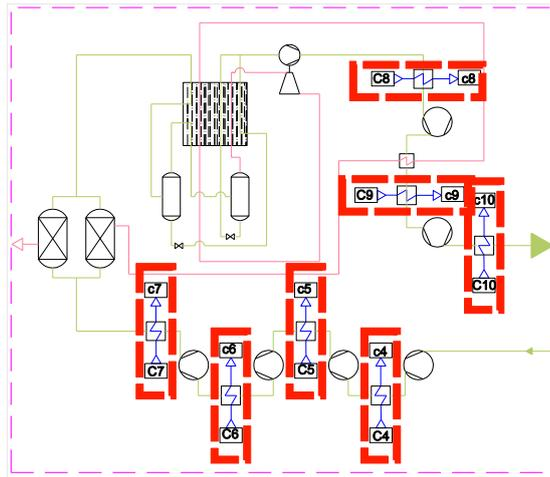
Figure 5: CO2 purification and compression unit with highlighted waste heat streams
