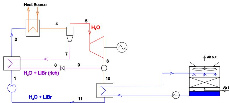
Figure 9: Schematic diagram of the LiBr Absorption Power Cycle
