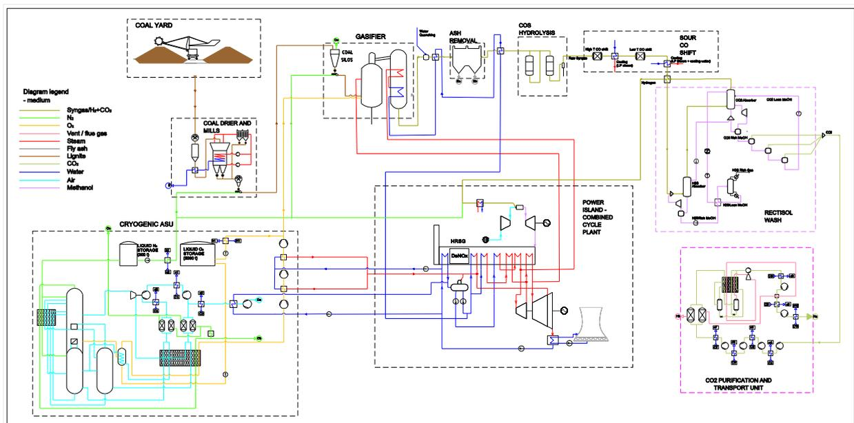
Figure 1: Process flow diagram of the base IGCC CCS plant
