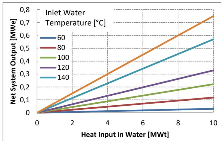
Figure 7: Net power output of potential WHR units
